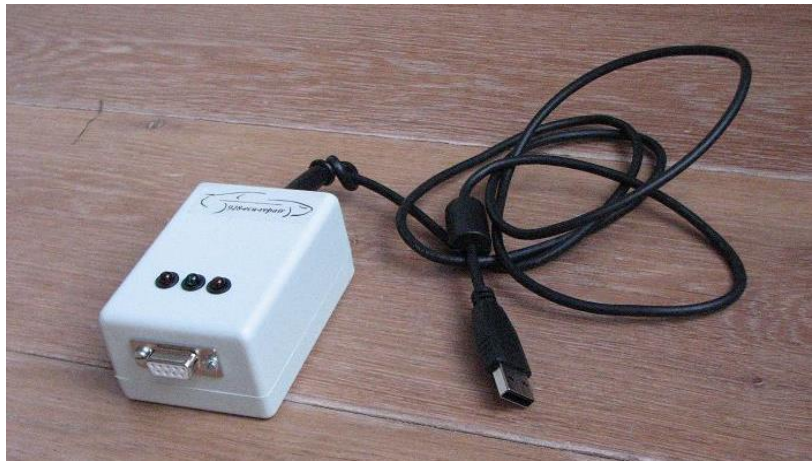
Model 2 ( \geq 2011 ): Interface module UDT999 with USB connection. This is the boxed design.
