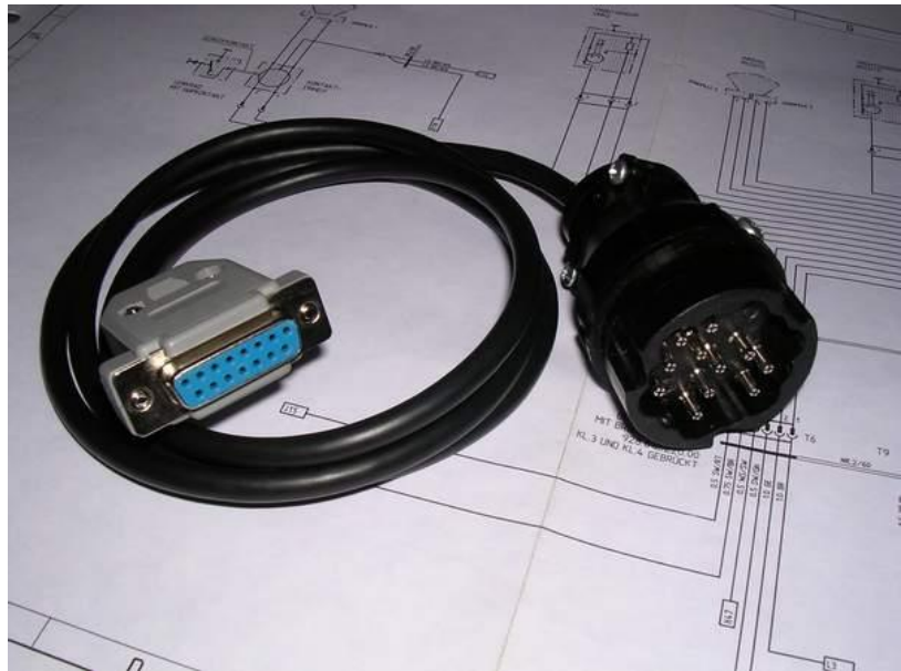
The interface cable DT9xx (model 1) to the 19pin diagnostic socket
