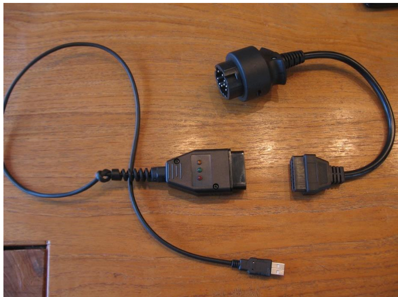
Model 2 ( \geq 2011 ): Interface module UDT999 with USB connection. This is the boxed design.
