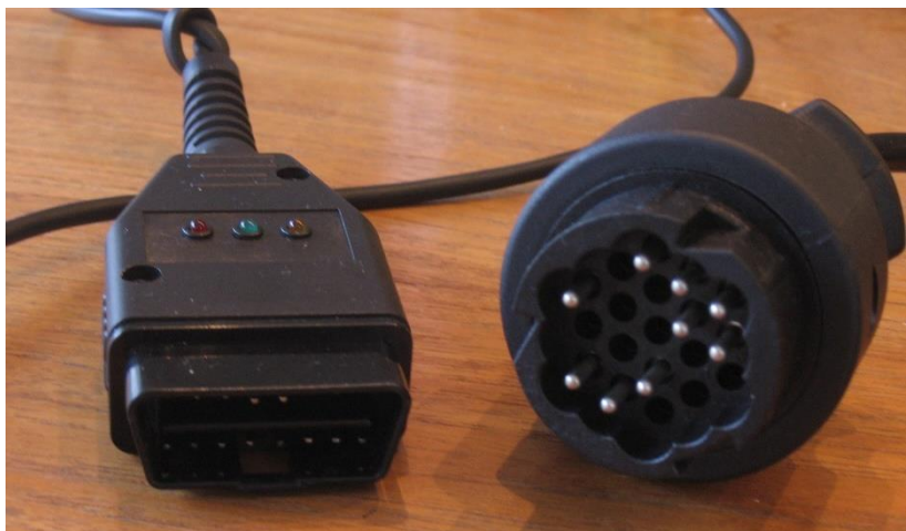
Model 3 ( \geq 2013 ): New style Interface module UDT999 with USB connection, OBD2 connection, and an OBD2 to 19pin OBD1 diag connector conversion cable.
