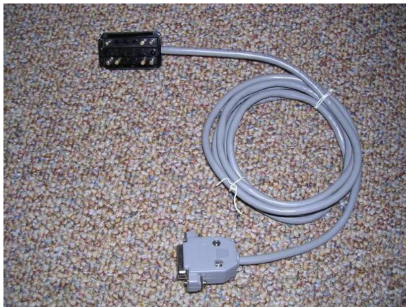
This is the 12pin diagnostic cable for the 1987/1988 Porsche 928 models and one 944S2.
